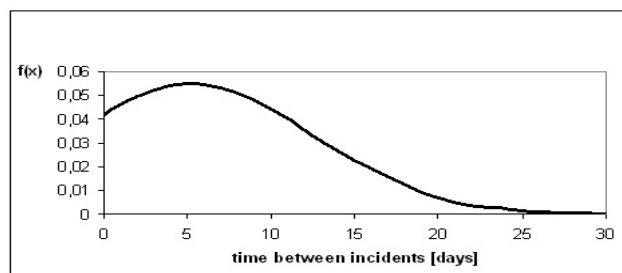
Figure 10. Probability distribution of observed time between the availability incidents. System B.
