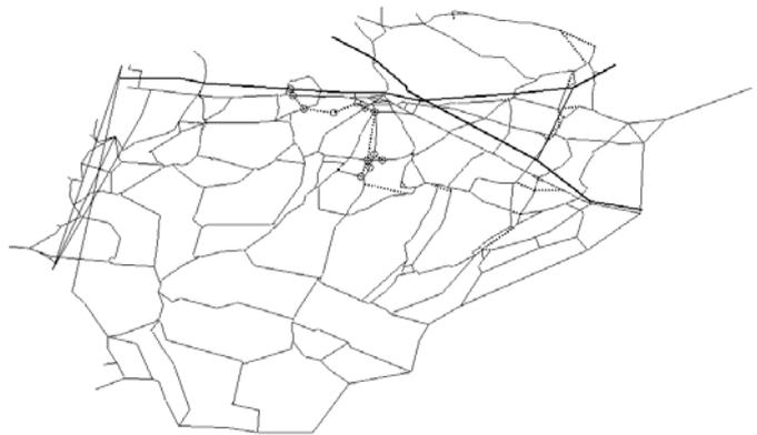
*Figure 4.* The road network with the bypass development plan: streets are drawn with dotted lines; the bypass is marked with circles.
