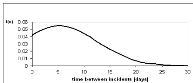
Figure 10. Probability distribution of observed time between the availability incidents. System B.
