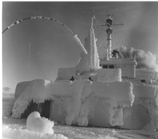
Figure 3. Example of icing in North Atlantic.(Photo: Kpt. Ź.W. Hieronim Majek)
