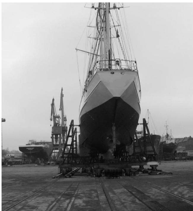
**Figure 4.** The ship during transportation from the traverser to the repair post R7.
