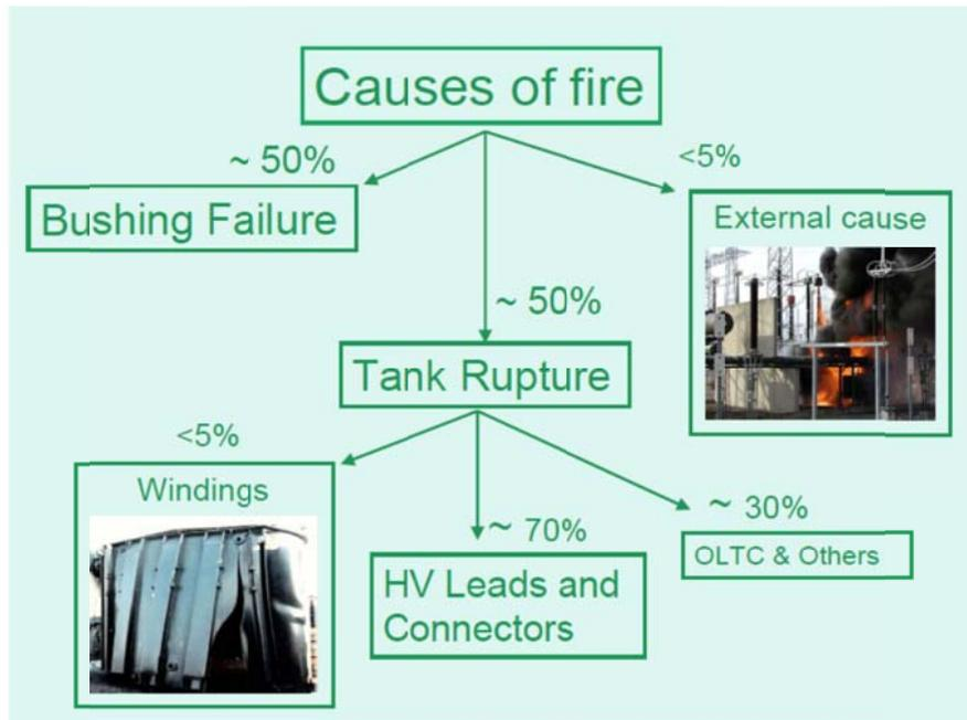
**Figure 6.** Causes of transformer fires (Foata 2010)
