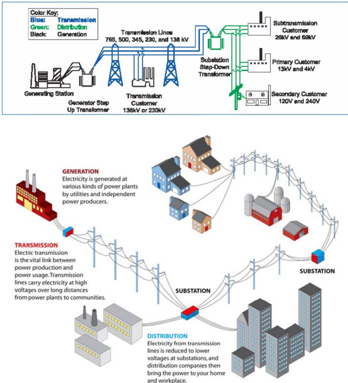
**Figure 1.** Typical electrical power network
