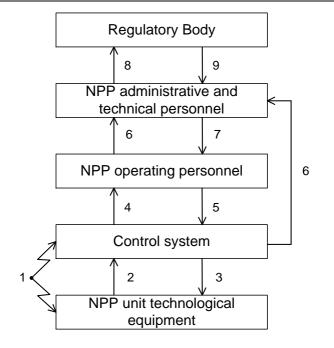
Figure1. General diagram of NPP unit safety control
