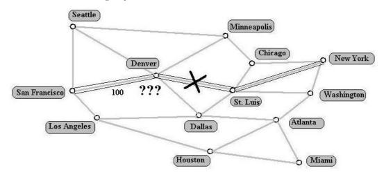
The model calculates new input data (loss of the trunk) and finds a new optimal traffic allocation between San Francisco and New York, taking into account minimum "harm" for other system users.
