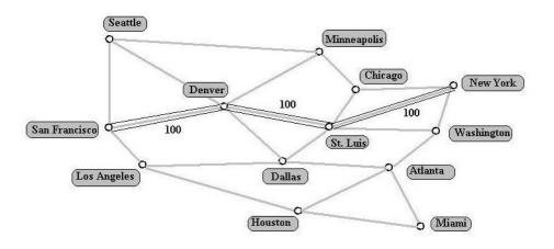
The model is working in interactive regime: a user would like to look at the network reaction on failure (or emergency turn off) of the trunk between Denver and St. Luis.
