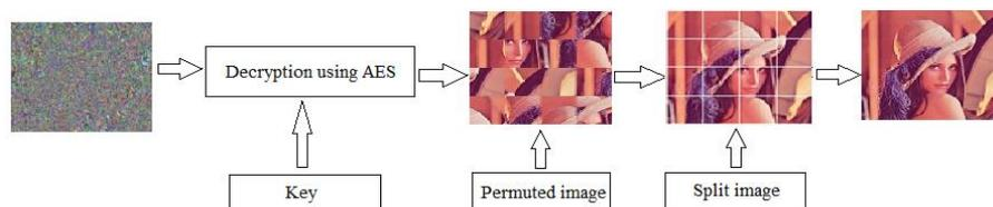
Figure 3: Block diagram of proposed decryption method
