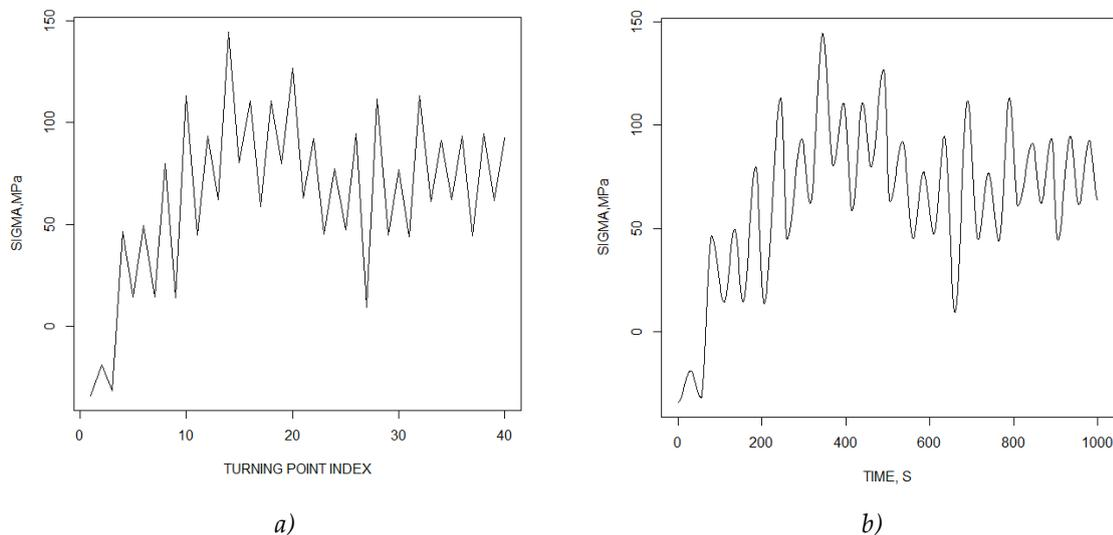
**Figure 4:** FALSTAFF (the beginning part) a) digit sequence of the turning points; b) continuous process, modelled by proposed method
