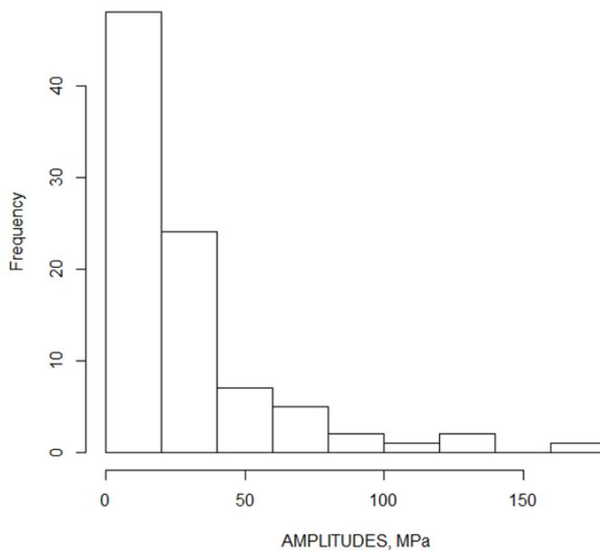
Figure 6: Rain-flow amplitudes histogram for the selected realization
