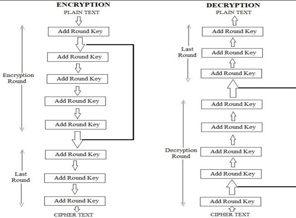
Figure 1: Encryption and decryption process of AES
