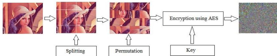
Figure 2: Block diagram of proposed encryption method
