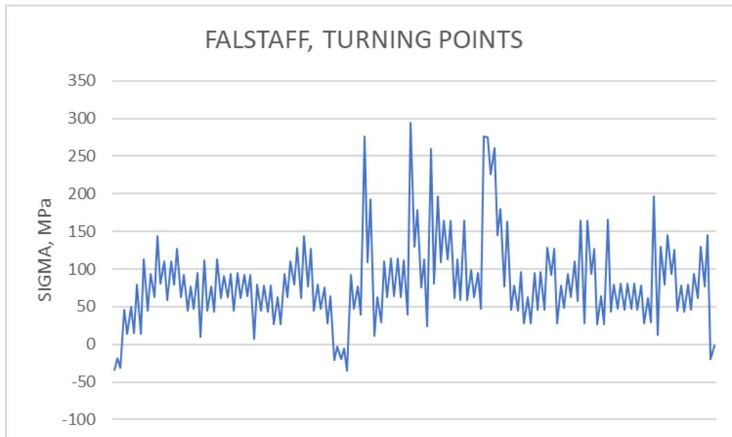
**Figure 1:** Digital sequence MIN-MAX-MIN-MAX ("the saw") of representation of the part of random loading process FALSTAFF in the working parts of a fighter airplane [4 Falstaff]
