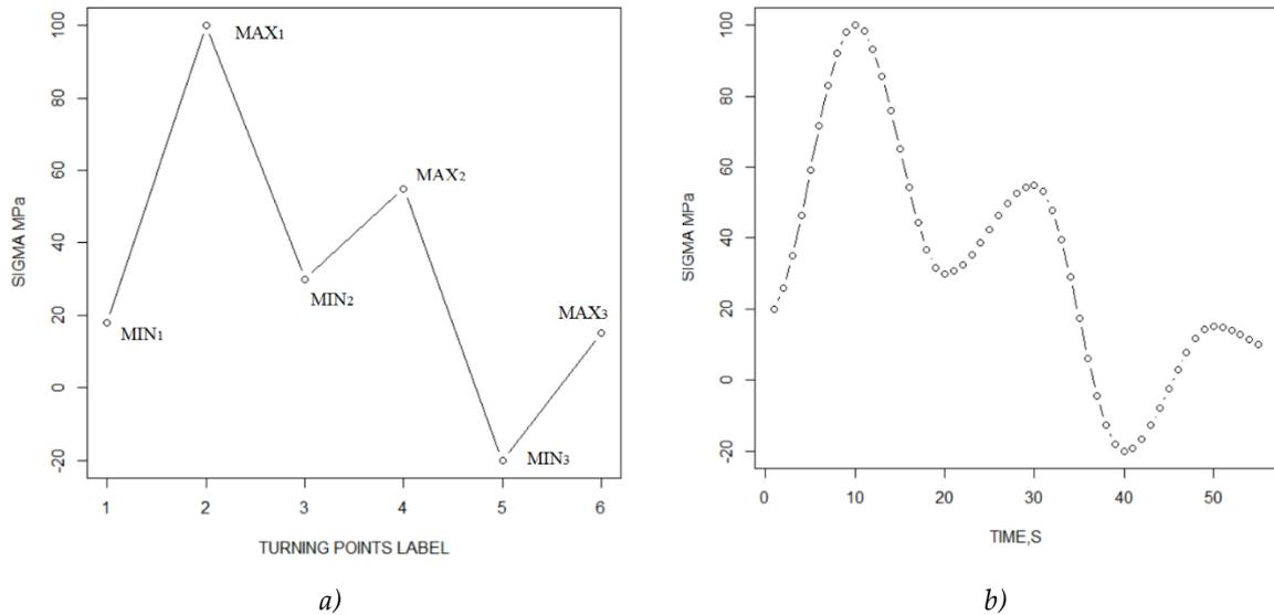
**Figure 2:** Cosine extrapolation of the short peaks sequence. 1a) initial data; 2b) extrapolation
