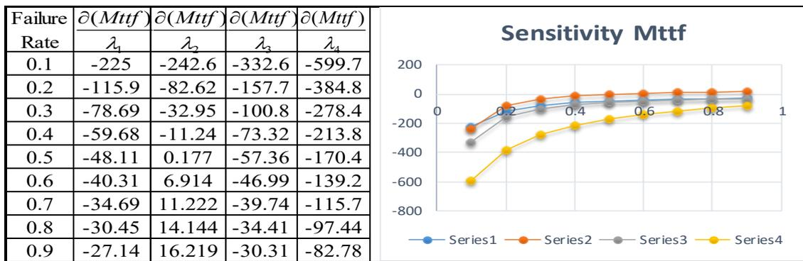
**Figure 5:** Sensitivity of MTTF as a function of failure rates
