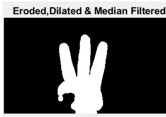
Figure: 6 Erosion, Dilation and Median applied to an image.
