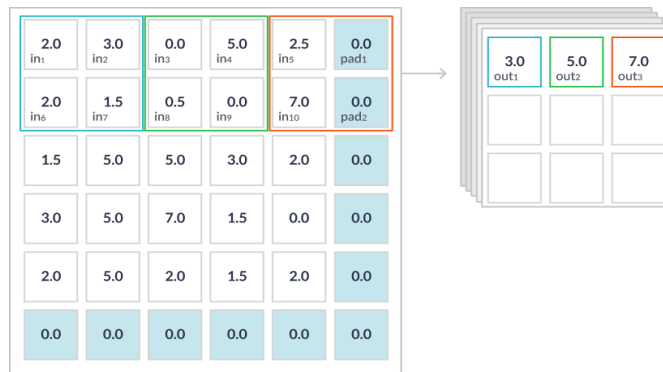
Figure 8: Maxpooling Method in CNN
