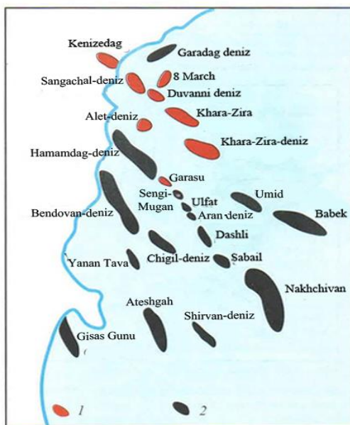
Figure 1: Location of structures within the Baku archipelago: 1 – identified oilfields; 2 – perspective structures
