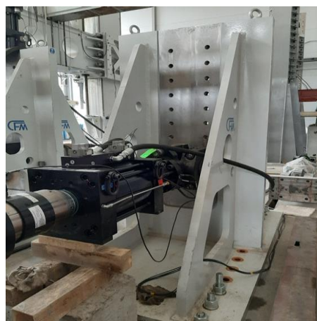
Fig. 6: Steel stops for hydraulic cylinders
