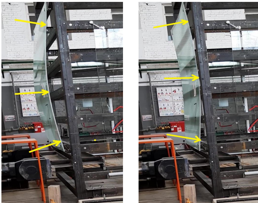
Fig. 8: Changing the geometry of the glass panel under dynamic influence
