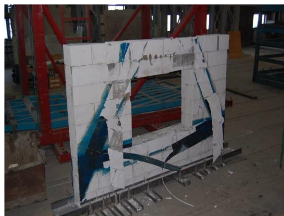
Fig. 12: General view reinforced with CFRP tapes after testing
