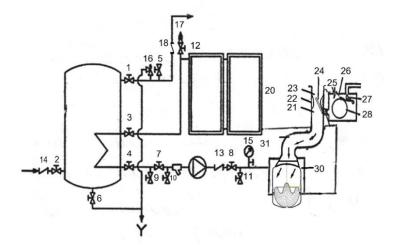
Figure 1: Schematic diagram of the proposed water heater
