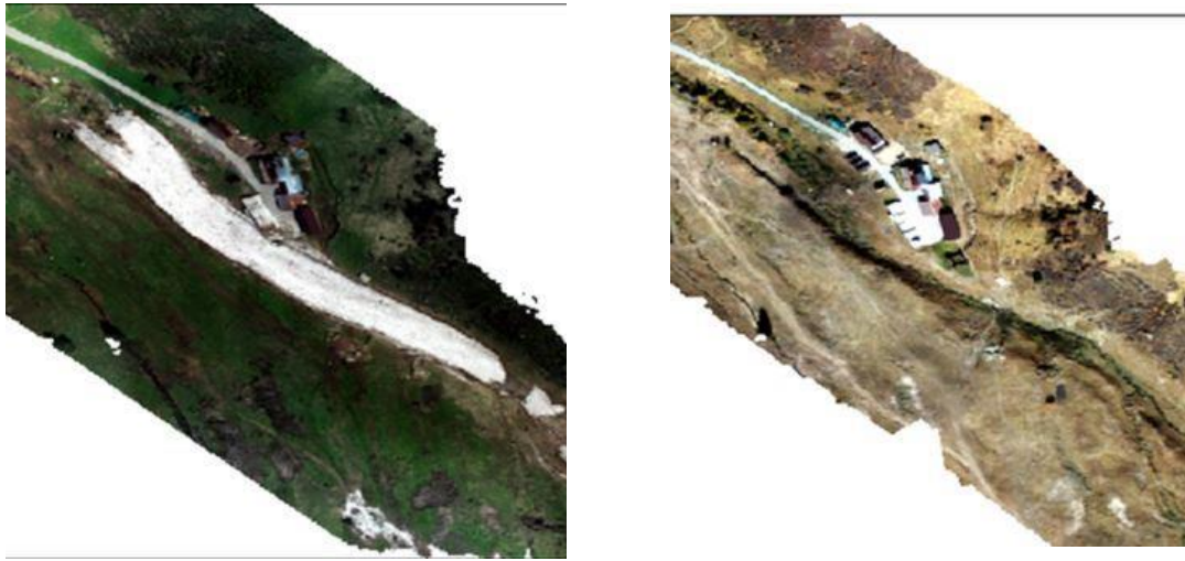
Fig. 3: Orthophotomaps of the area with and without avalanche snowpack near the "Pioneer" campground
