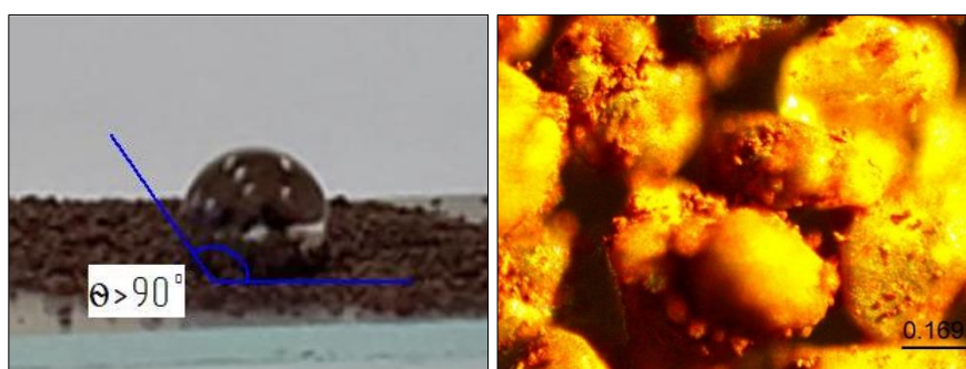
Fig. 3: Microphotos of modified glauconite: left – contact angle of wetting of hydrophobic glauconite for oil spill response; right – globules of glauconite coated with nanomagnetite
