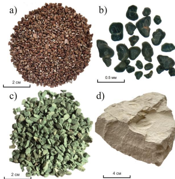
Fig. 1: Photographs of natural mineral sorbents: a – vermiculite, b – glauconite, c – zeolite, d – diatomite.
