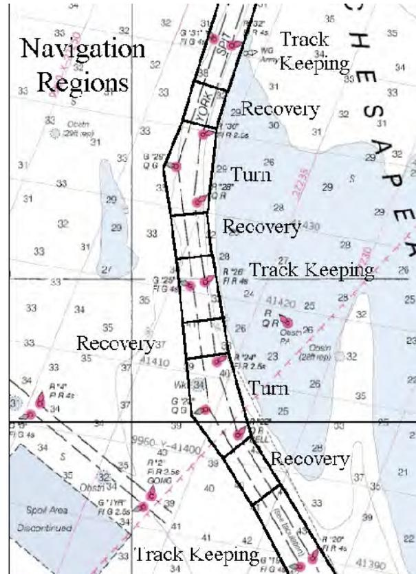
Figure 1. The vessel manoeuvring phases (IALA NAVIGUIDE 2006).
