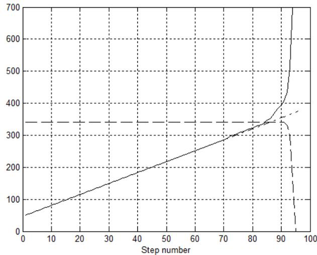
Fig. 6. DS (-), the residual strength (--) and process of loading (-.) for tensile strength test.
