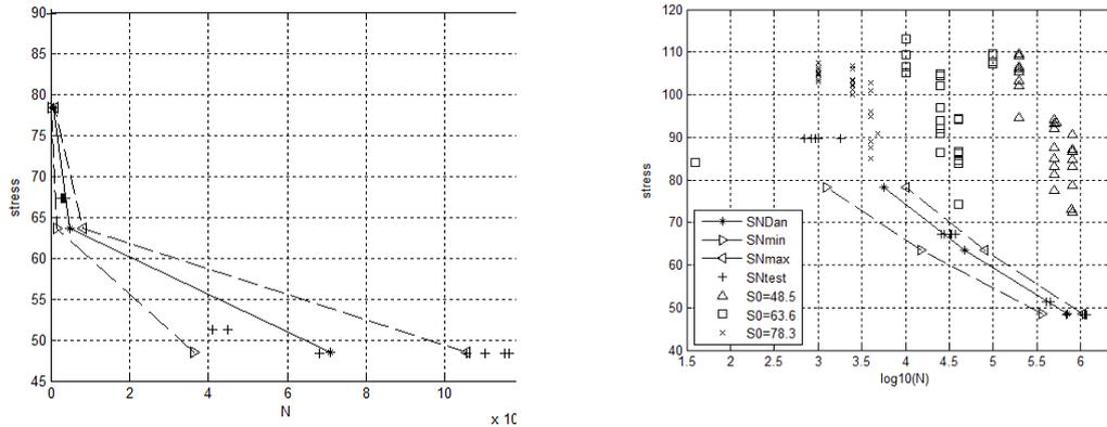
**Fig.3.** The test result (+), calculated mean (\*) and the extrem values (►, ◄) corresponding to two standard deviation from mean value. The test residual strength for preliminary load levels 48.5 MPa, 63.6 MPa and 78.3 MPa for 20%, 50% and 80% of the corresponding nominal life time.
