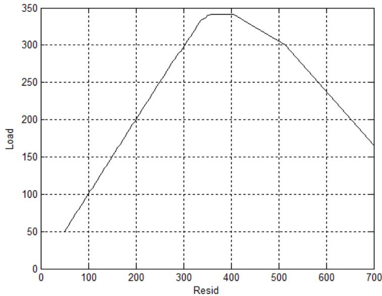
Fig. 7. The curve "the load versus residual strength" is similar to stress-strain curve in static strength test
