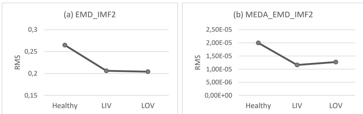
Figure 2: RMS value of IMF2 extracted with (a) EMD and (b) MEDA-EMD method for healthy, LIV and LOV states
