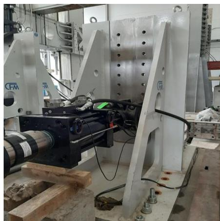
**Fig. 6:** Steel stops for hydraulic cylinders
