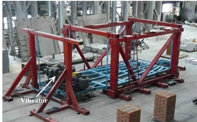
**Fig. 1:** *Pendulum type vibration platform*
