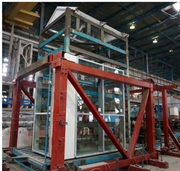
**Fig. 2:** *Glass facade mounted on a vibration platform*
