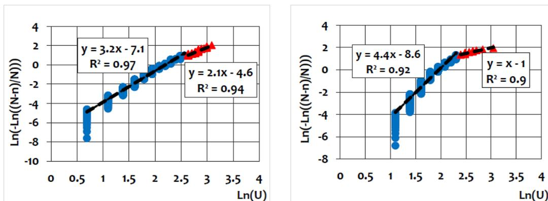
**Figure 3:** Empirical distributions of extreme wind speeds of the year (1966 - 2013) according to measurements at Lovozero (left) stations during cold periods and Okunev Nose (right) during warm periods, constructed in the coordinates of the Weibull probability distribution, where the line segments correspond to two different laws of distribution.
