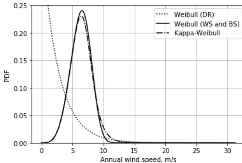
**Figure 8:** PDF of extreme wind speeds according to measurements at Okunev Nose station (summer period) corresponding to three families of Weibull distributions: "WS and BS", "DR" and  $\kappa$ -deformed
