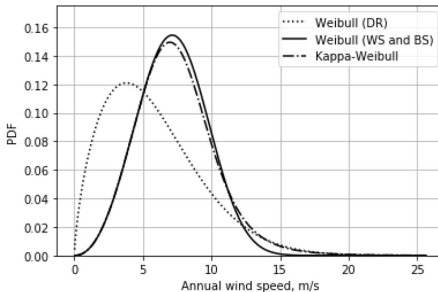
**Figure 9:** PDF of extreme wind speeds according to measurements at Lovozero station (winter period) corresponding to three families of Weibull distributions: "WS and BS", "DR" and  $\kappa$ -deformed
