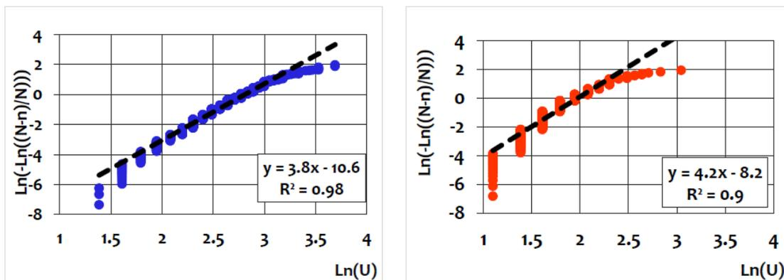
**Figure 2:** Empirical distributions of extreme wind speeds (1966 - 2013) according to measurements at Teriberka station (left) in cold periods and at Okunev Nose station (right) in warm periods of the year, plotted in the coordinates of the Weibull probability distribution
