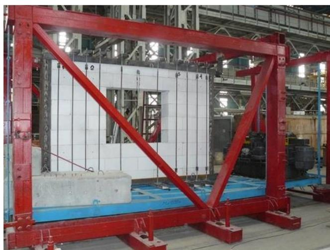
Fig. 8: Samples I series on the vibration platform
