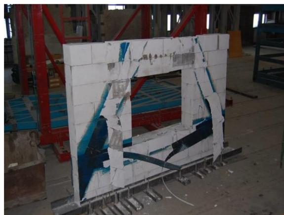
**Fig. 12:** *General view reinforced with CFRP tapes after testing*
