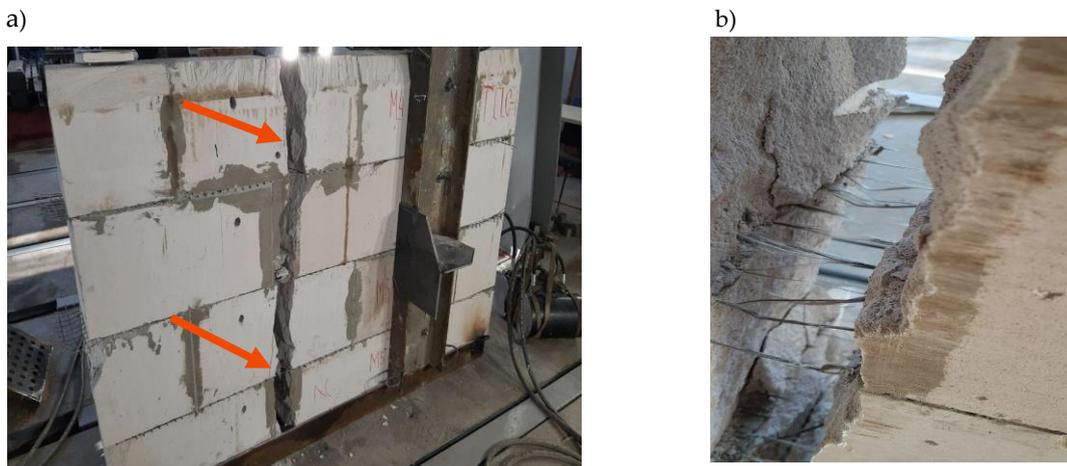
**Fig. 13:** *The nature of the destruction of the reinforced sample during stretching*
