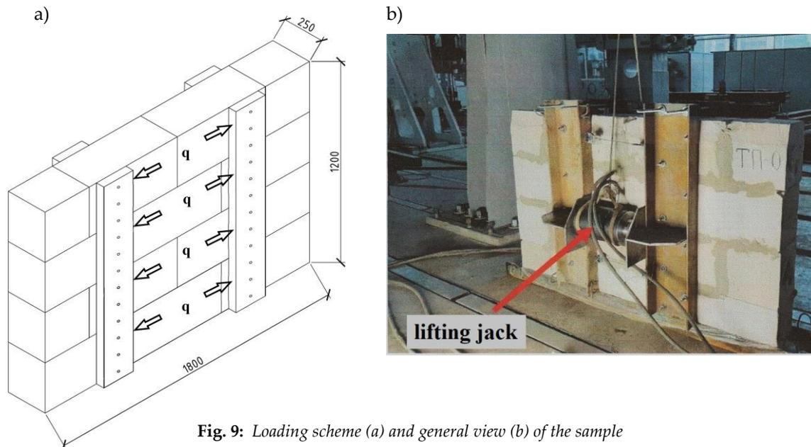
Fig. 9: Loading scheme (a) and general view (b) of the sample
