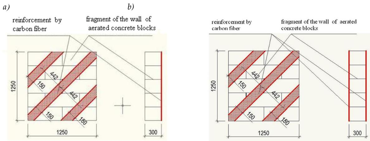
Fig. 3: Samples of the II (a) and III (b) series
