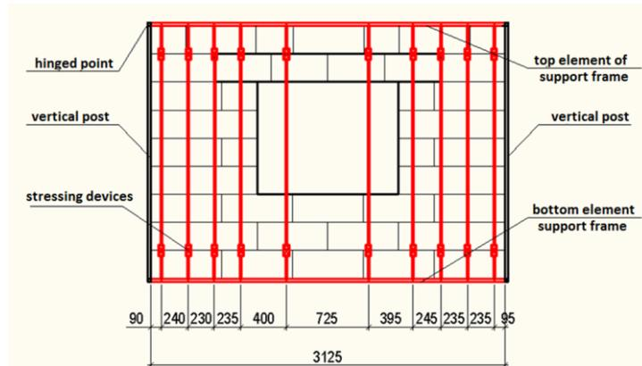
Fig. 6: Device for creating a vertical load
