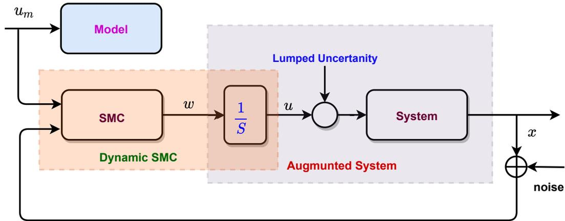
Figure 1: Model following DSMC design with measurement noise
