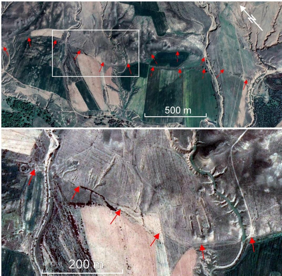
**Fig. 5:** The Kura fault sections at  $41.097^{\circ}$  N,  $45.74^{\circ}$  E with 4-5 m high scarp marked by red arrows, optimal for trenching (T-2 in Fig. 2). The lower image is the zoomed fragment outlined above. The indubitable fault scarp is marked by solid arrows, the assumed section – by dashed arrows
