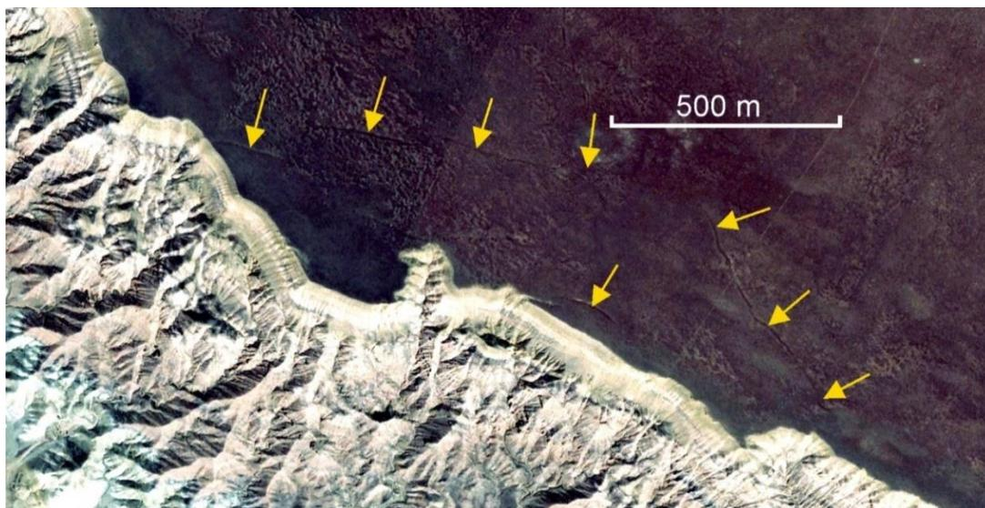
**Fig. 7:** Fissured indicating the initial stage of the deep seated gravitational slope deformation on top of the ridge (Ls-2 in Fig. 2). Fractures are marked by orange arrows. Image made on April 5, 2014
