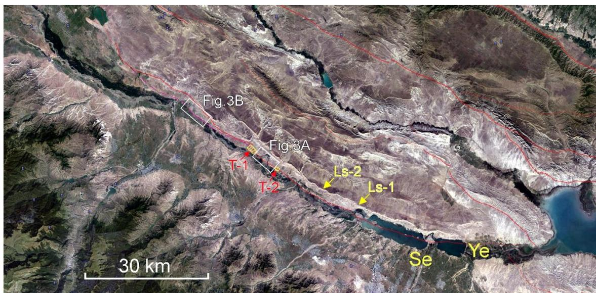
**Fig. 2:** Space image of the area marked in Fig. 1. Red lines – active faults according to the EDAF. Pink lines specified position of the Kura active faults. Ye – the Yenikend HPP, S – the Şamkir HPP, white rectangles – fault sections shown in Fig. 3A and B; T-1 and T-2 – sites most suitable for trenching shown in Figs 4 and 5; arrows marked by Ls-1 and Ls-2 indicate sites with deep seated gravirational slope deformations shown in Figs. 6 and 7
