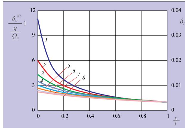
Fig. 3. Detection of the leakage degrees in the initial point of pipe:
