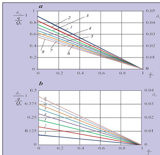
**Fig. 2:** Detection of the leakage area and degree by the relevant change of discharge (a) and pressure (b):
