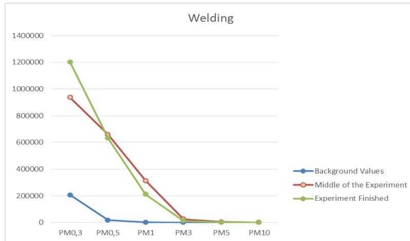
**Fig. 3:** Graph of the quantitative composition of airborne particles in the ambient air during underwater welding
