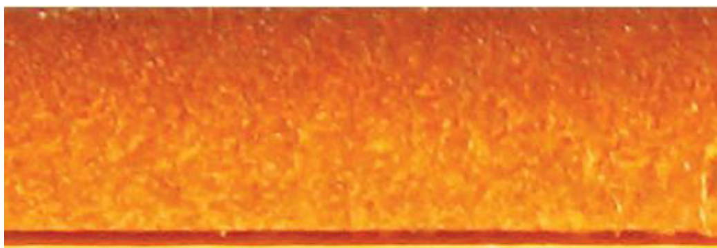
Figure 1:. Side surface a cut in a copper workpiece 2 mm thick
