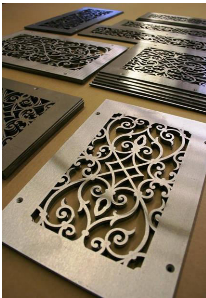
Figure 4: Example contour cutting a part made 63 brass with a thickness 2 mm
