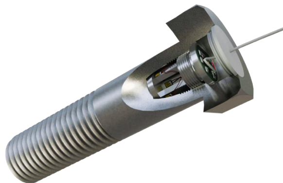
Figure 6: Sensor-integrating screw of the project SiSmaK [21]
