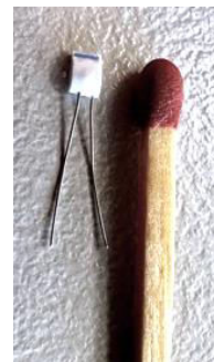
Figure 8: PT100 temperature sensors idler in size comparison with a match [24]
