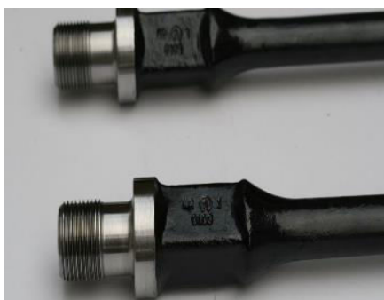
Figure 1: Head and transition zone of pump rods ShG-19 and ShG-22
