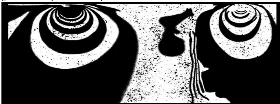
Figure 1: Isochromes under loading of an isotropic material (left) and a material containing solid inclusions (right). Load 150 kg; E_{ucl} = 46000 ; E_{max} = 16000
