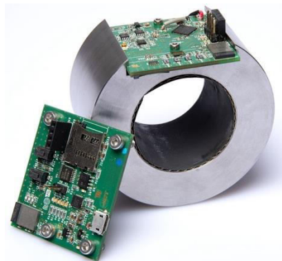
Figure 4: Gas foil bearing with the first version of the sensor system [16]
